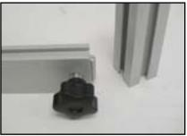
Detail F: Plastic Star Knobs are used to tighten locks where horizontal extrusions connect with vertical extrusions. Turn the knobs clockwise to tighten. Turn counterclockwise to loosen, but do not remove knob.
