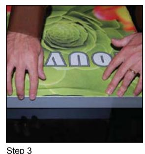
Once all corners are inserted, press one silicon edge into channel from corners and work toward the center. Make sure welt is fully inserted into channel. Continue until all sides are done. Smooth out edges of graphic.
