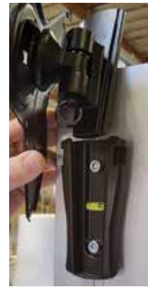
Slide monitor mount into back piece.
